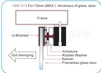
Application for the Electromagnet: 10001 Series 10005 Series (Double)
